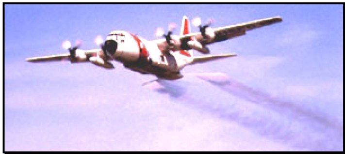
A Coast Guard C-130 fitted with a modular dispersant system sprays water in a May 1997 exercise in Oregon
